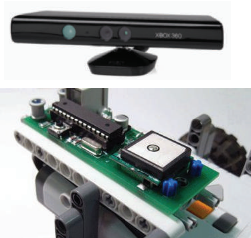
Fig. 1.4 Some additional sensors that we could use such as the Microsoft Kinect and a GPS for the Lego NXT.
