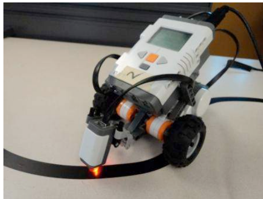
Fig. 4.1 Basic Lego Robot with microprocessor, two motors, and a light sensor.
